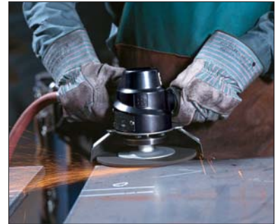
88V / 99V series vertical grinders Available with motor power from 1.50 to 2.25 kW and wheel capacities from 150 to 230 mm.
